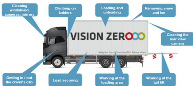
Figure 1. Hazards when working with commercial vehicles
